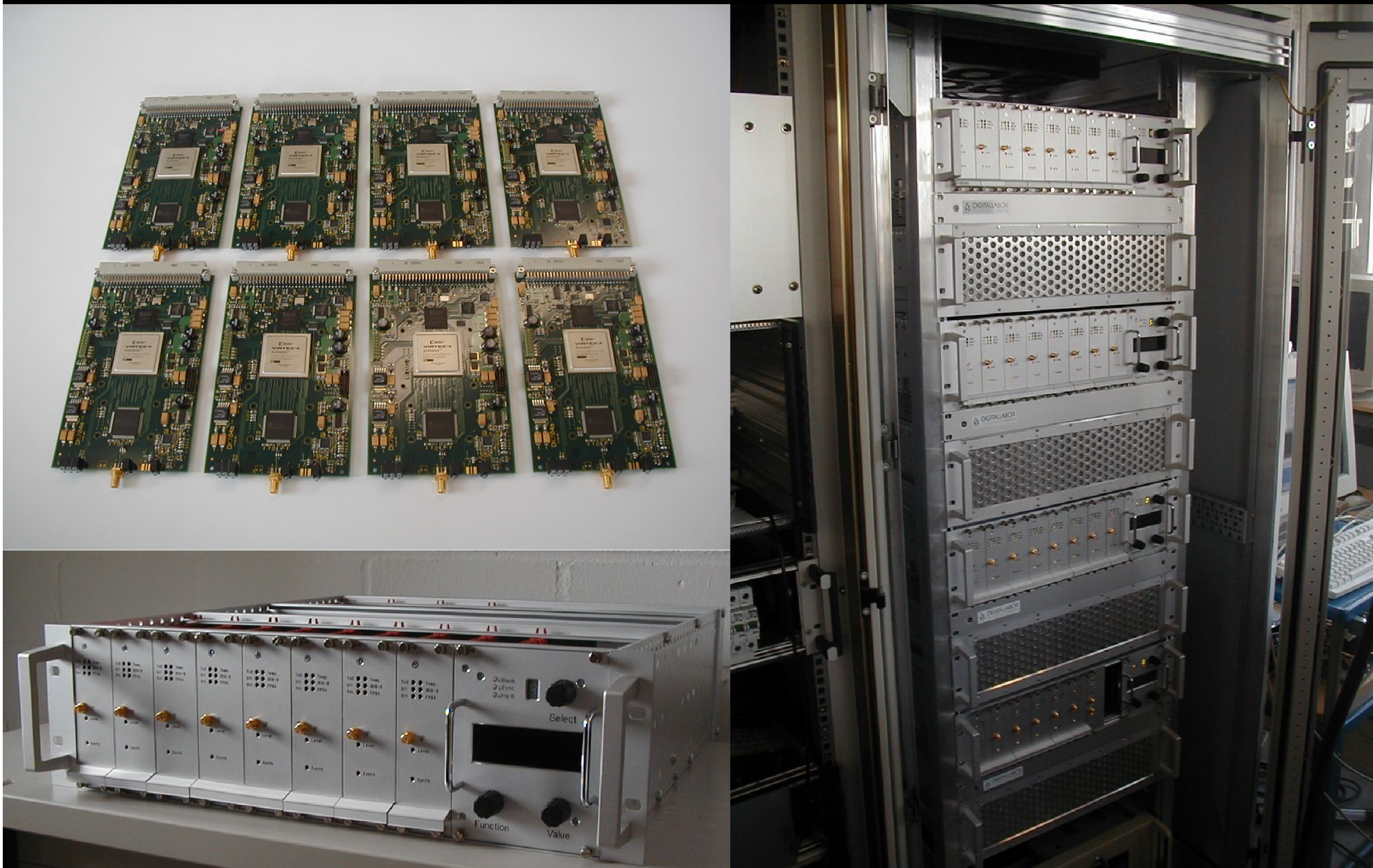
APEX Array Fast Fourier Transform Spectrometer: 4 \times 8 \times 1.5 \text{ GHz} = 48 \text{ GHz}/262144 channels
